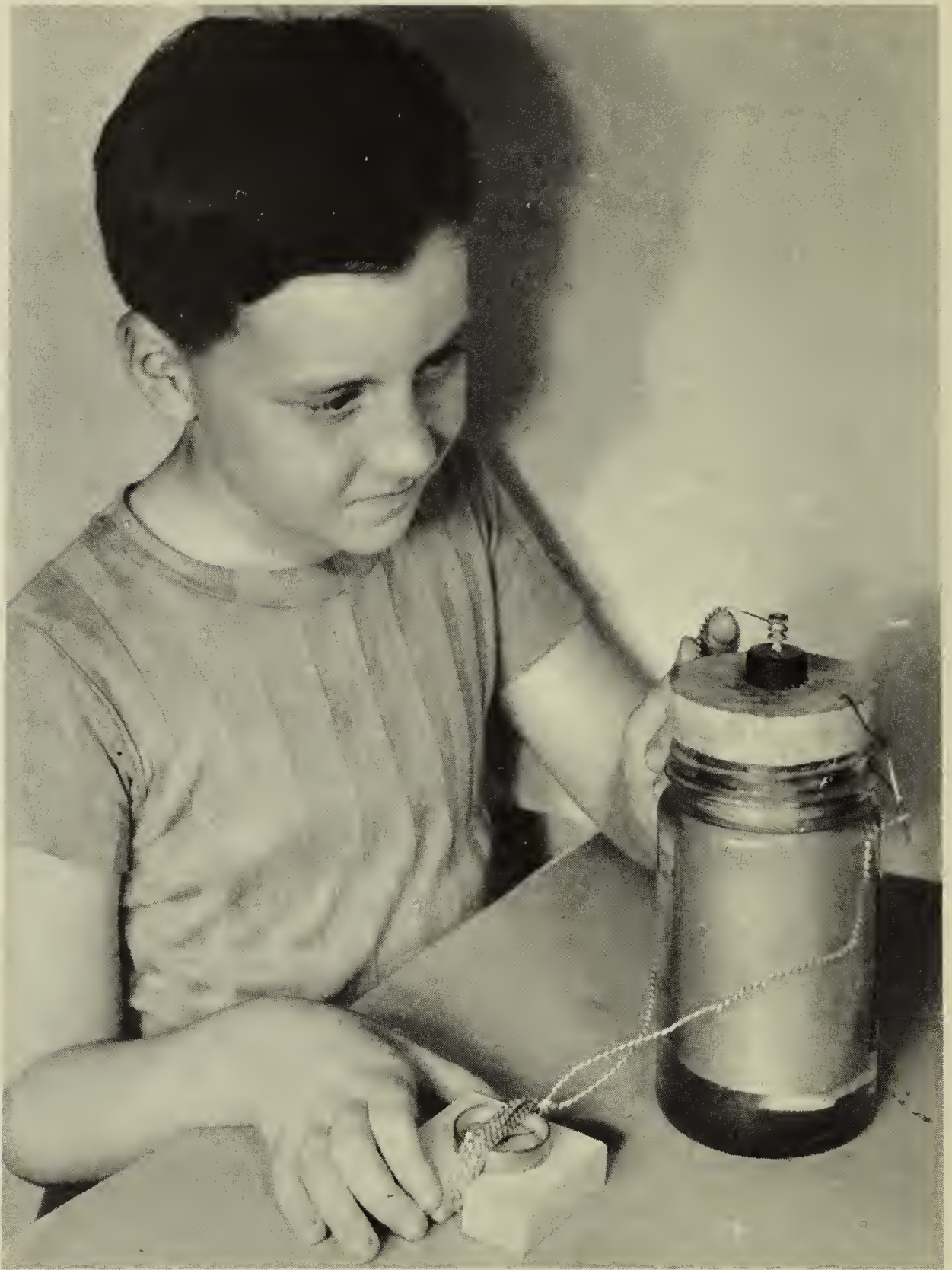
Fig. 11. The current detector being used to test an electric cell.
